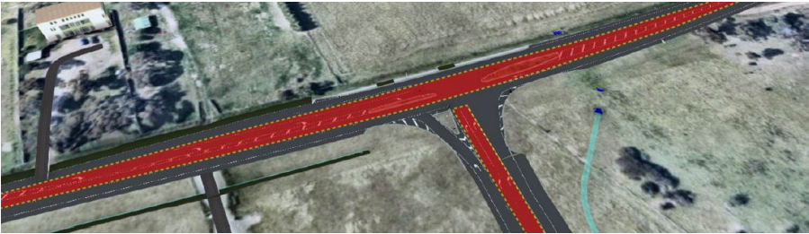
Stage 3: Traffic lanes will be divided, with a central work zone established
