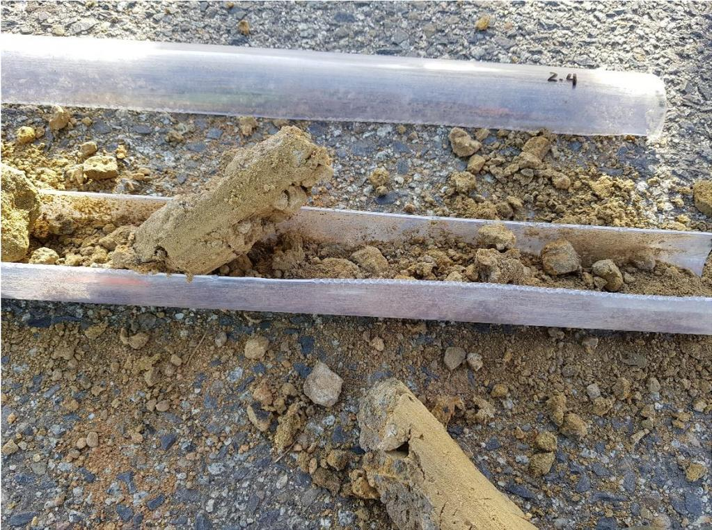
**Photo 4. Weathered basalt gravels.**
