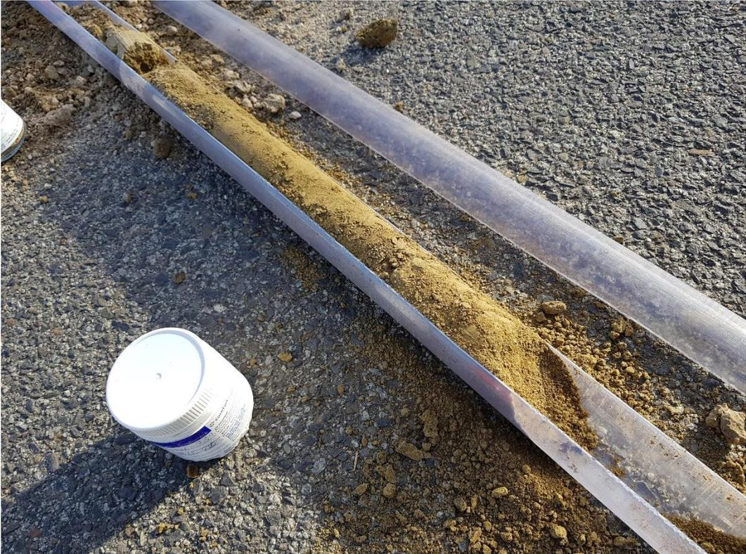
**Photo 3. Orange-brown sandy clay material encountered beneath silty clay at some locations.**
