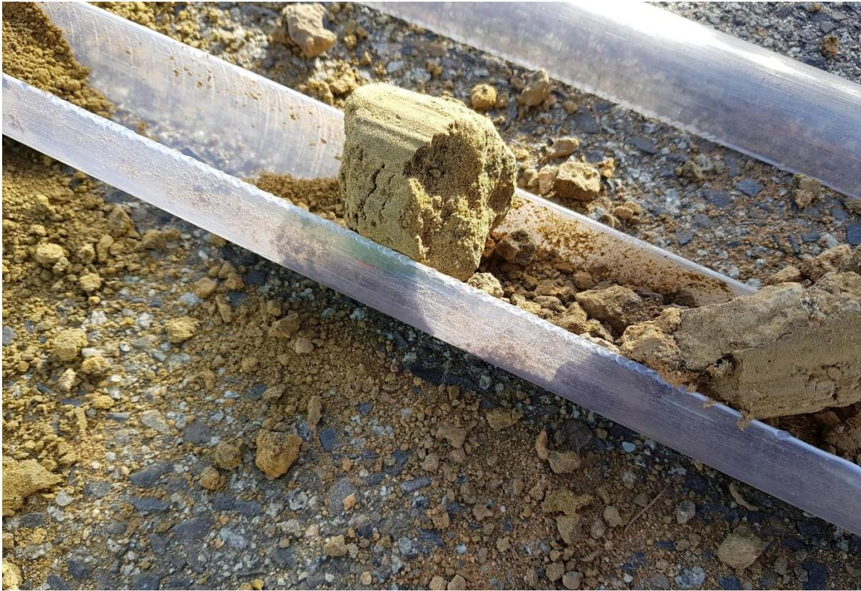
**Photo 5. Orange-brown clayey sand with basalt gravels encountered within some locations.**
