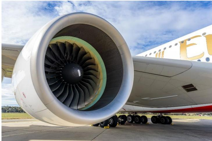
Engine ingestion is when an aircraft engine draws an object into itself. When the engine is operating it creates a low-pressure area in front of the engine. This low-pressure area causes a large quantity of air to rush into the engine inlet area.
