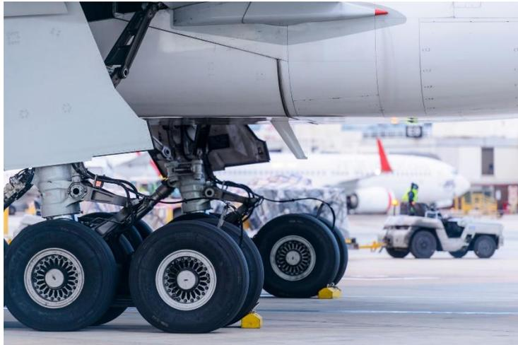
As well as the landing gear, there are many other components located in the wheel wells of an aircraft. The landing gear struts, wheels, brake assemblies and even an auxiliary power unit in the case of some aircraft types.
