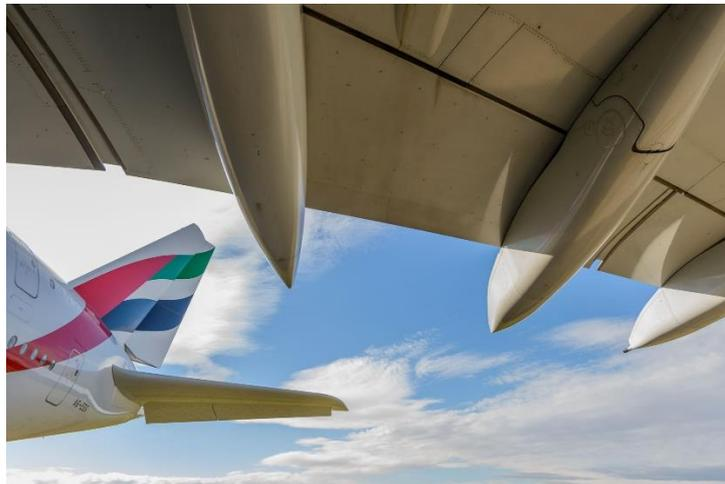
The underwing area contains many of the aircraft flight controls including the flaps, the engines and the cowlings.
