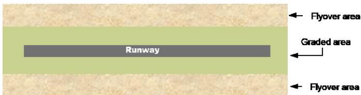
Figure 1: Composition of a runway strip
